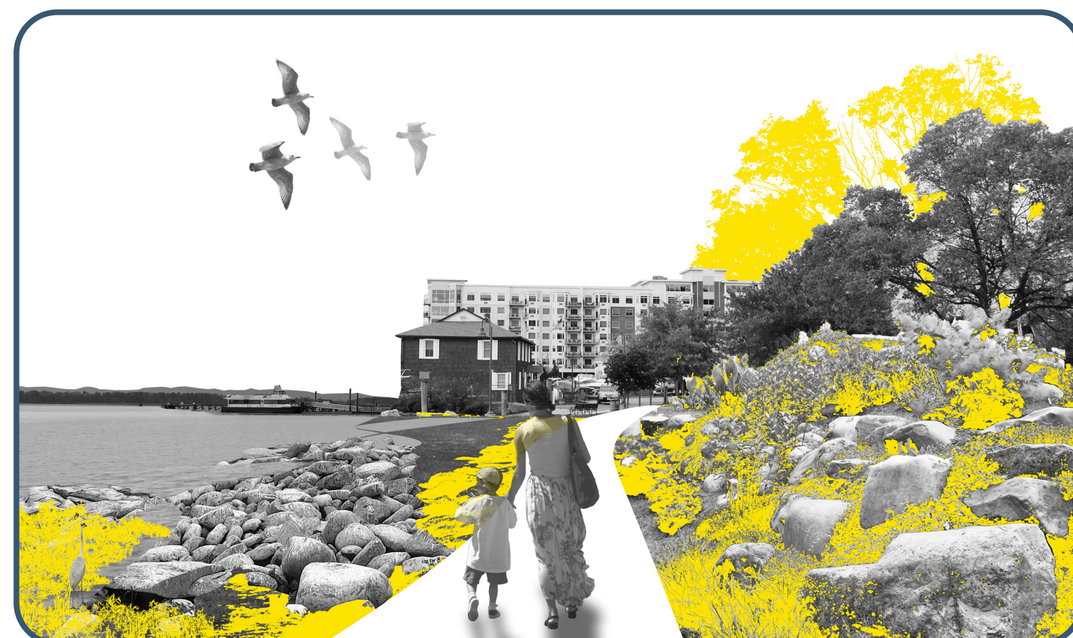
View of a sustainable shoreline that mixes vegetation with large boulders to prevent erosion, enhance habitat and provide aesthetic value.
